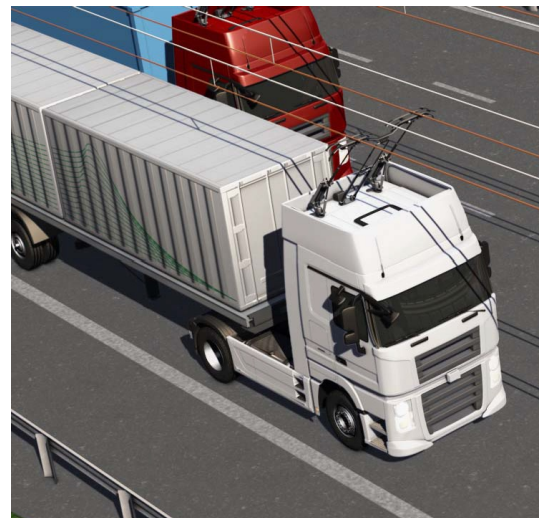
Figure 10. Catenary truck concept drawing (source: Siemens Mobility)
