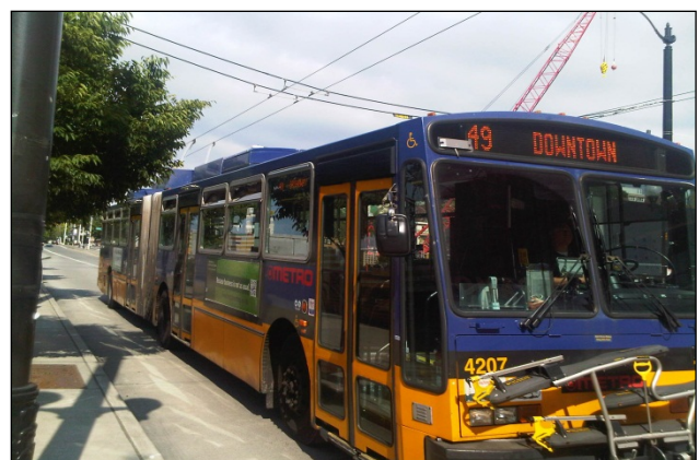
Figure 7. Catenary hybrid diesel bus (King County METRO)
