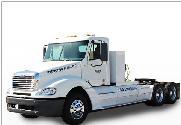
Figure 5. Fuel cell hybrid truck (source: Vision Motors)
