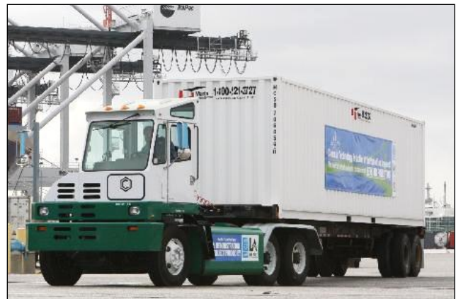
Figure 6. Battery electric truck (source: Balqon)
