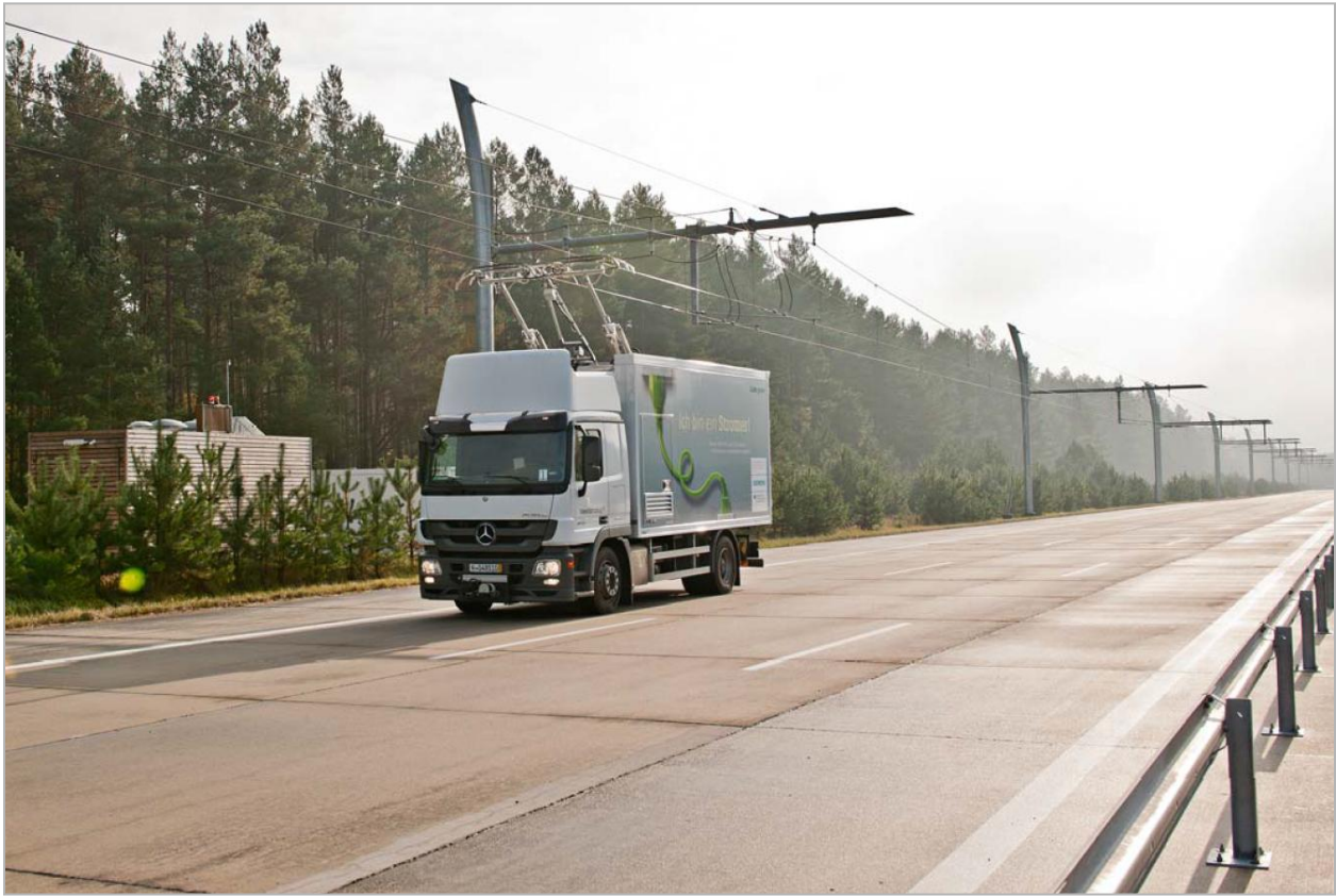
Figure 16. Siemens catenary hybrid truck in operation (source: Siemens Mobility)
