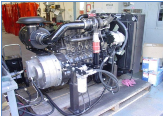
Figure A-1 – Engine integrated with hybrid system
