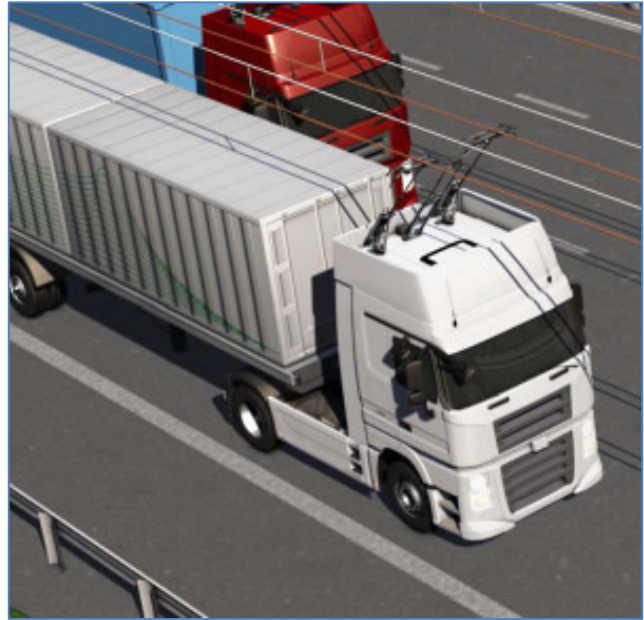
Figure 14 – Artist's rendering of the Siemens – Transpower catenary/natural gas drayage truck (Source: Siemens)
