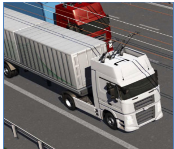
Figure A-5 – Siemens catenary truck concept (Source: Siemens)
