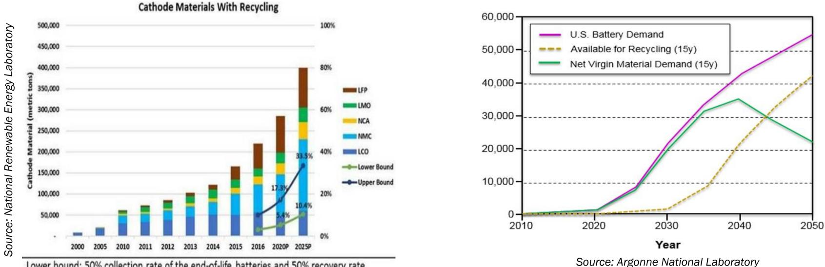
Lower bound: 50% collection rate of the end-of-life batteries and 50% recovery rate Upper bound: 90% collection rate of the end-of-life batteries and 90% recovery rate Percentages represent potential of cathode materials demand filled by recycled materials
