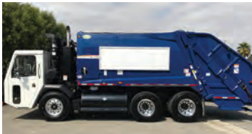
Crane Carrier: Hybrid-Electric Refuse Truck w/ Active Stop-Start Tech - Ultra Low NOx NG Engine
