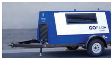
Onboard Dynamics: GoFlo CNG80 Mobile Natural Gas Compressor
