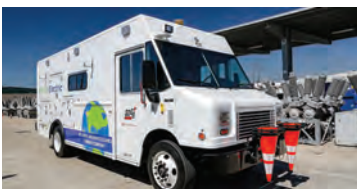
Odyne Systems: Worksite Electrification System (ePTO) on FCCC Chassis
