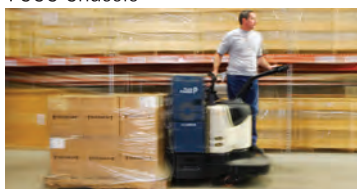
Plug Power: Plug Power GenDrive Fuel Cell-Powered Pallet Jack
