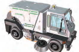
US Hybrid: Class 7 Electric Street Sweeper
