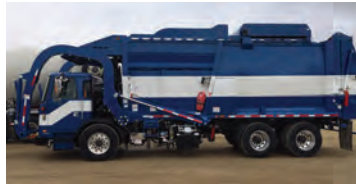
Autocar Truck: Front Loader Refuse Truck w/ L9N CNG Engine
