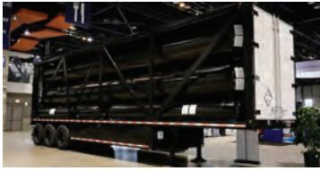
Hexagon Composites: 40-foot TITAN XL CNG Transport Trailer
