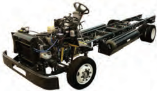
Agility: Freightliner Custom MT45 Strip Chassis w/Agility Low-NOx GM 6.0L NG Engine; Agility CNG Fuel Storage System
