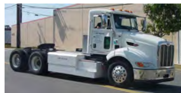
US Hybrid Plug-In Hybrid-Electric/LNG Class 8 Tractor
