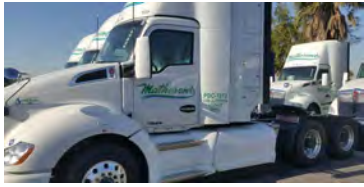
Kenworth T680 ISX12-G with Agility CNG Fuel Cabinet System
