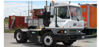
Effenco Hybrid-Electric Yard Truck with Active Start/Stop Technology
