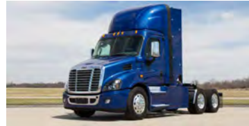
Agility Fuel Solutions - Freightliner Cascadia Class 8 Tractor with CNG Agility Fuel System
