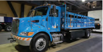
PG&E Plug-In Hybrid-Electric Class 6 Truck w/CWI 9-Liter NZE Engine
