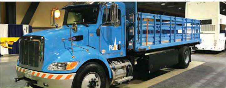
PG&E Unveiled its new plug-in electric hybrid class-6 truck that features exportable power capacity of up to 160kW that can power up to 125 homes.
