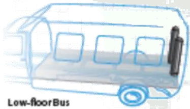
Low-floor Bus Two vertically-installed rear tanks for rear exit door.
