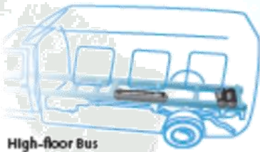
High-floor Bus Three below-floor tanks - 40 gal. - 32 gal.
